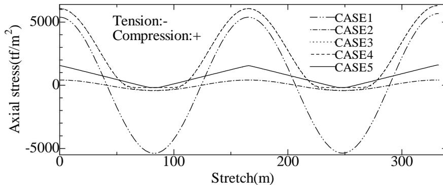
Figure 9 : Axial stress distribution of shield tunnel
