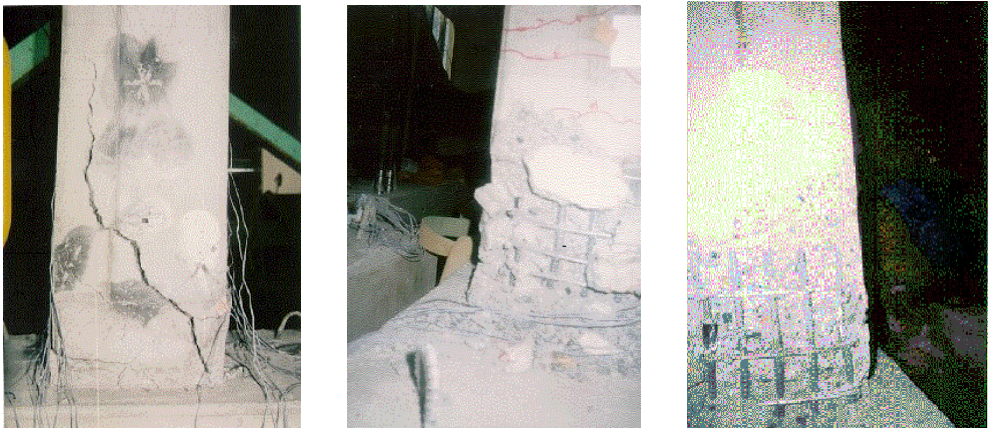
Figure 8: Photos 1, 2 and 3 for final failure mode of tested specimens B, D and H respectively. Shear Reinfnt.=0.115%. Shear Reinfnt.=0.236%. Shear Reinfnt.=0.472%.
