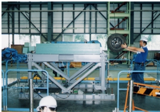
Figure 15 Test Frame with Damper
