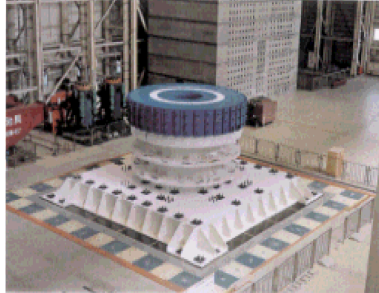
Figure 2 : A Typical Example of RC Structure Test by Applying Dynamic Load
