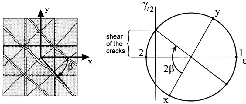
Fig. 7 - Strains due to deformations at the cracks
