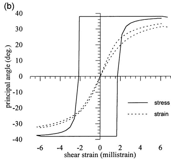
Fig. 4 - Principle angles, cyclic case: (a) experimental (SE8); (b) proposed model
