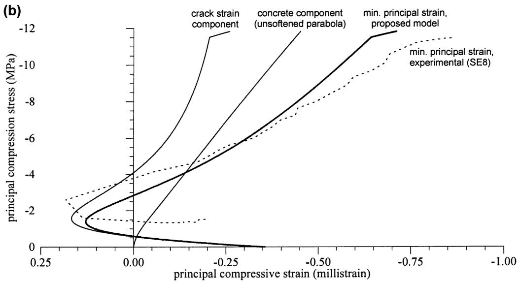
Fig. 8 - Concrete response: (a) monotonic; (b) cyclic
