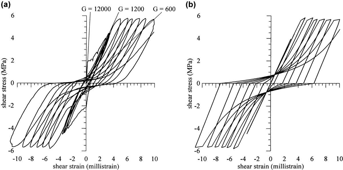
Fig. 1 - Shear response of specimen SE8: (a) experimental; (b) predicted
