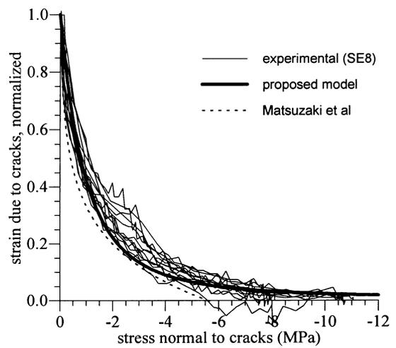
Fig. 6 - Crack closing relationship
