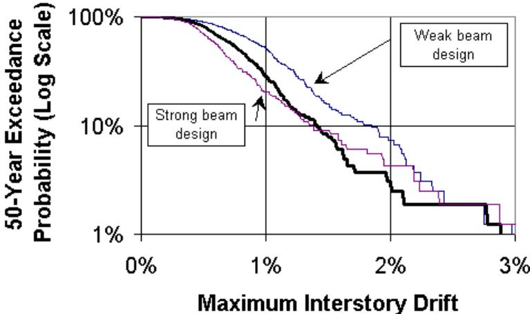
Figure 6. Results of Simulation Study Presented in the Two-Dimensional Performance Space.
