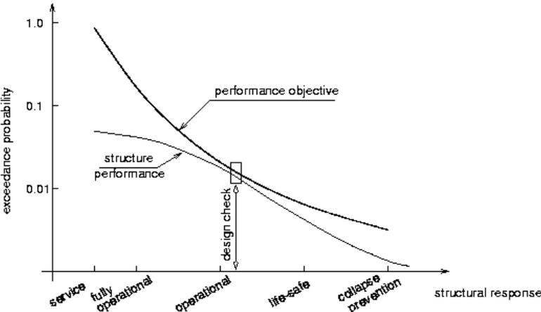
**Figure 5. PO and SP Curves with Opposite Concavity.**
