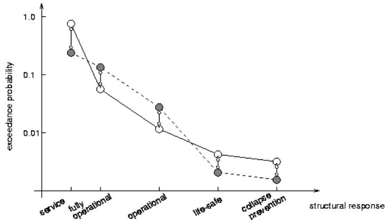
**Figure 2. Effect of a Change of Code Performance Objectives on the Shape of the PO Curve.**
