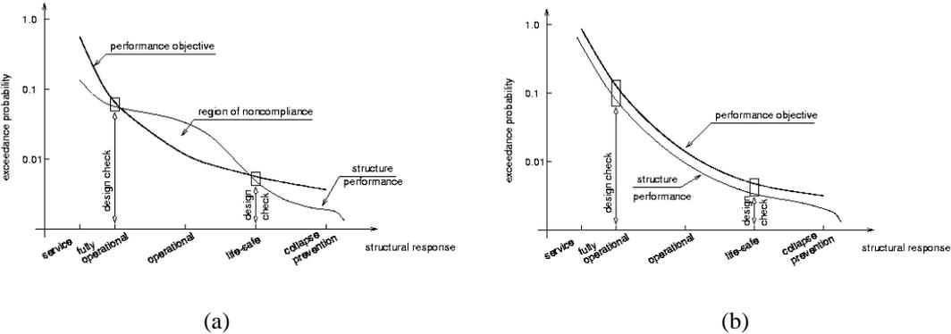
**Figure 4. Possible Scenarios for a Two-Point Design Check. (a) Incompatible PO and SP Curves. (b) Compatible PO and SP Curves.**
