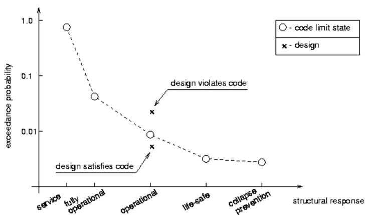
Figure 1. Reliability-Based Definition of Performance Objectives.
