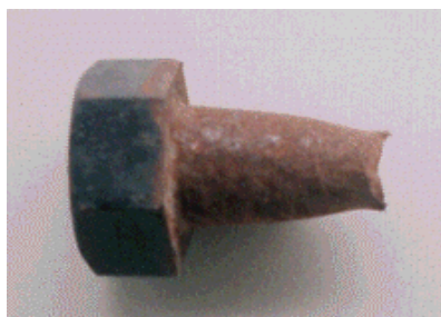
(b) Ruptured set-bolts
