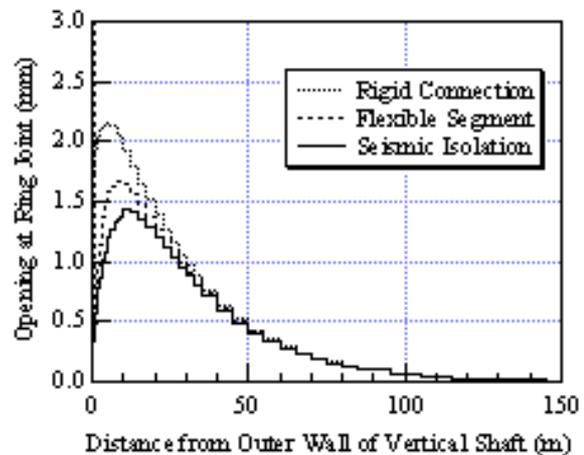
Figure 14: Comparison in opening of ring joints among three different cases
