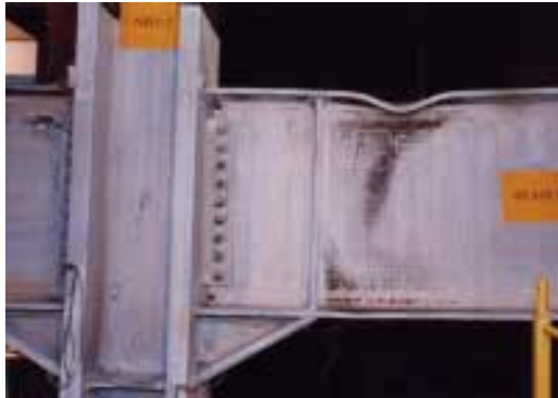
(a) Deformed Configuration of NIST-2
