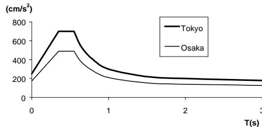
**Figure 4: The mean values of maximum response spectrum,  $S_A(T)$ , in 50 years (from Saito et al. [1998])**
