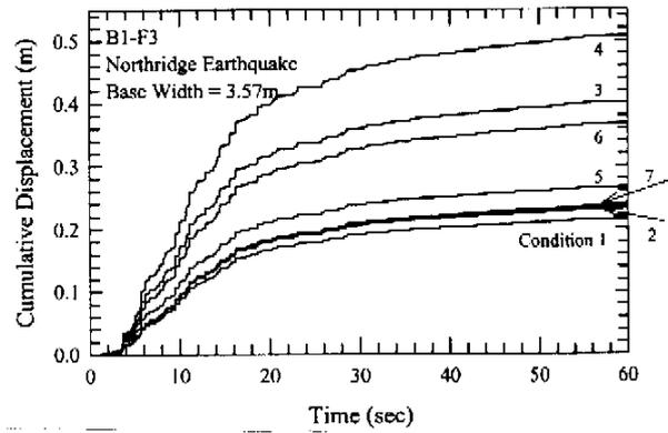
Figure 2. Computed displacements for 6m high wall (B1-F3) for conditions 1-7
