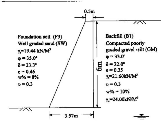
Figure 1. Dimensions of wall and soil properties in foundation (F3) and Backfill (B1)
