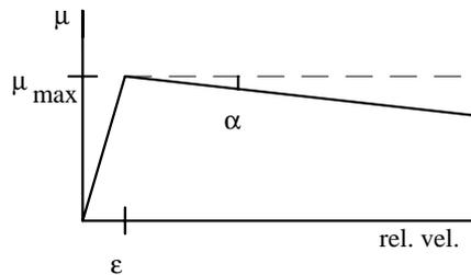
**Figure 2: Modelling of friction coefficient**
