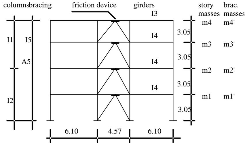
**Figure 1: Four story frame (dimensions in meters)**
