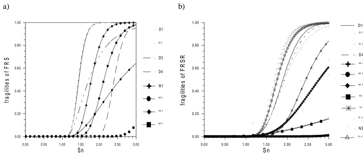
Figure 6: Fragilities on normalized seismic intensity
