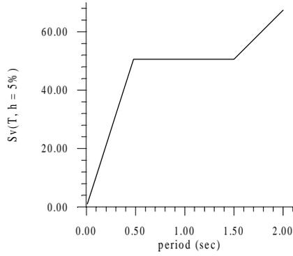
**Figure 3: Target response spectrum**
