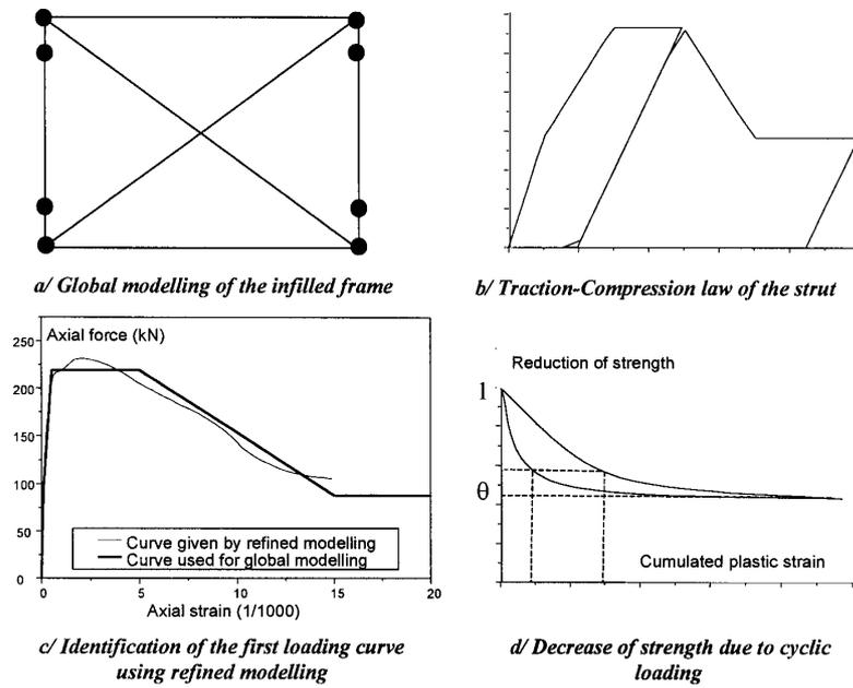
**Figure 2 – Global modelling of infilled frames**
