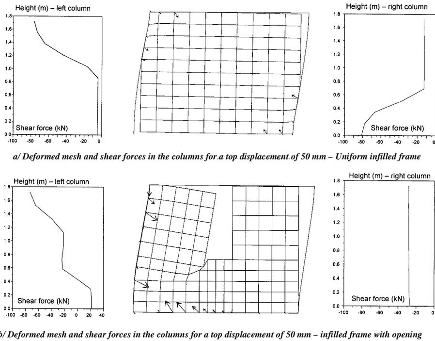
Figure 3 – Deformed mesh and repartition of shear forces in the surrounding frame (refined modelling)
