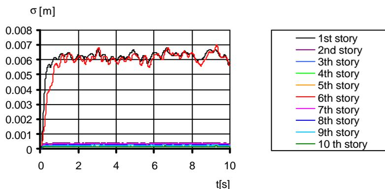
**Figure 5: Standard deviations of story drifts over time for 10 story building with SLs in every 5<sup>th</sup> story.**
