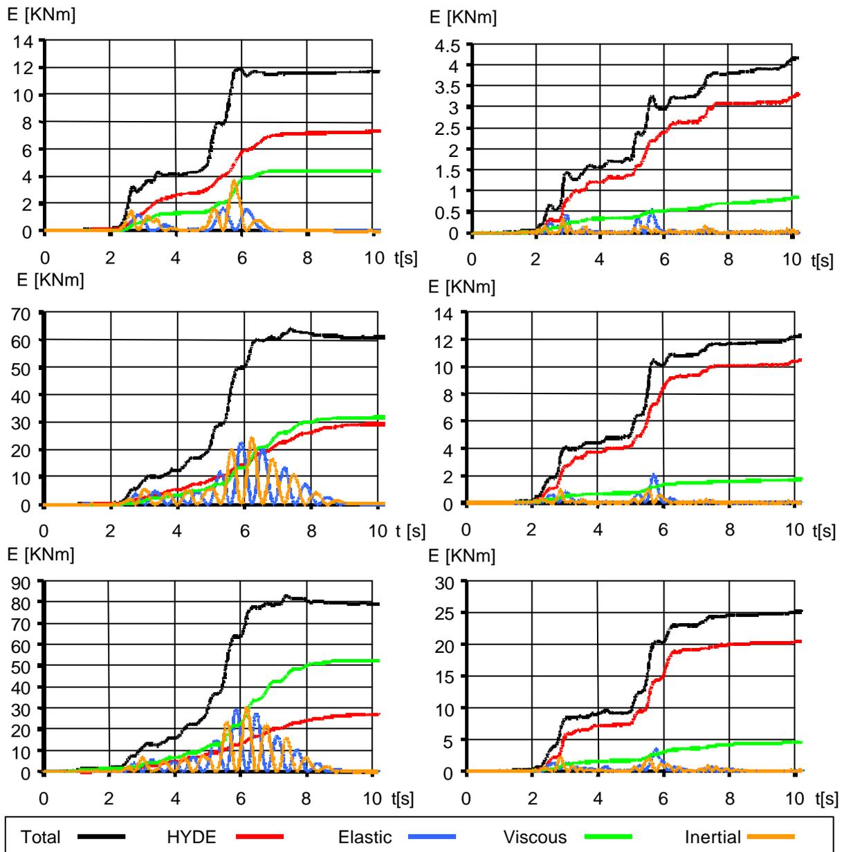
**Figure 6: Energies over time in the 5- (above), 10- (middle) and 15 story buildings (below) with SLs in each story (left) and every 5<sup>th</sup> story (right).**
