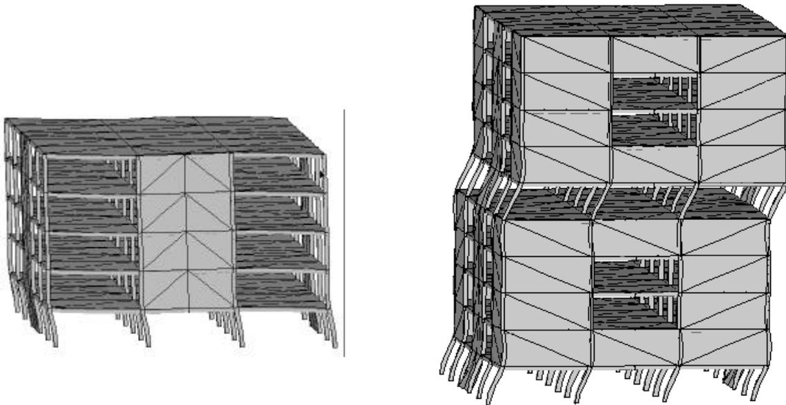
**Figure 4: 3D finite element models of 5 and 10 story structure: Deformed states (scale factor 50).**
