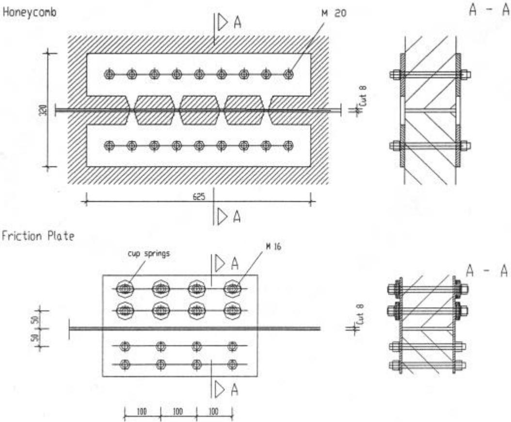
Figure 3: Two types of simple Hydes based on yielding and friction.
