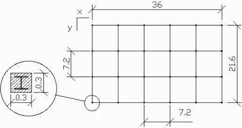
Figure 2: Ground plan of office buildings. Measures are in meters.
