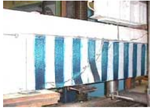
(b) Specimen C-BT5 (Debonding of CFRP below shear crack)
