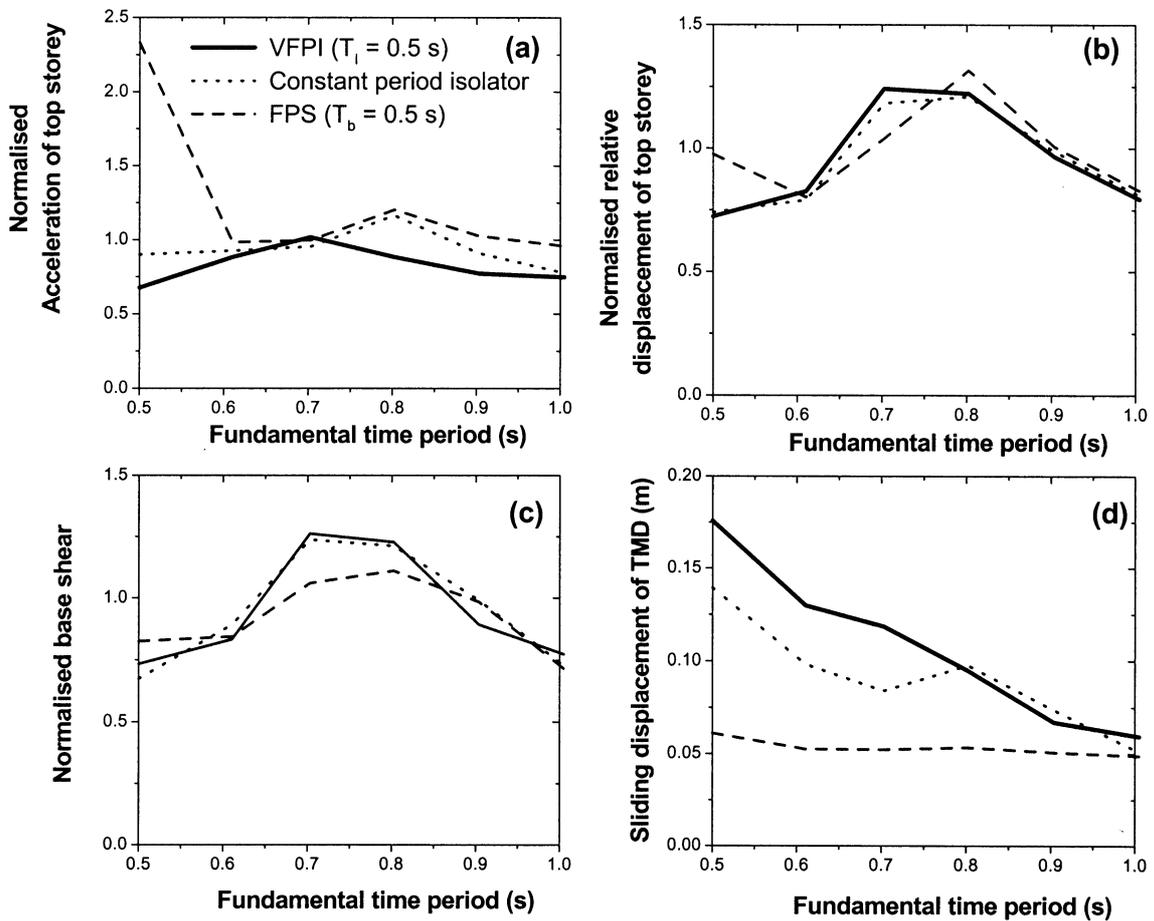
Figure 4. Structural response of example building with TMD subjected to El Centro 1940(NS) ground motion ( $T_I = 0.5$ s, FVF = 1.0,  $\mu = 0.02$ ,  $\xi = 5\%$ ).
