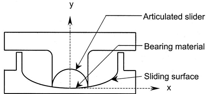
**Figure 1. Schematic view of a VFPI, showing the main components.**
