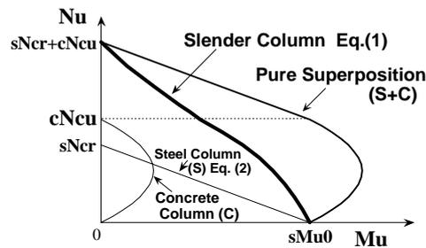
Figure 5: Superposed strength
