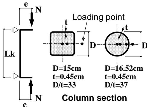
Figure 1: Loading condition (Series I)
