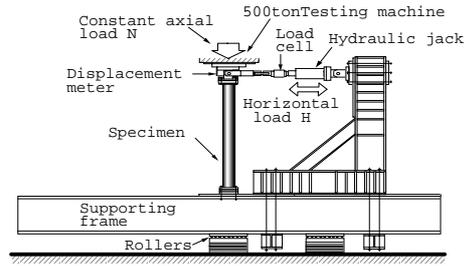
Figure 4: Loading apparatus (Series II)
