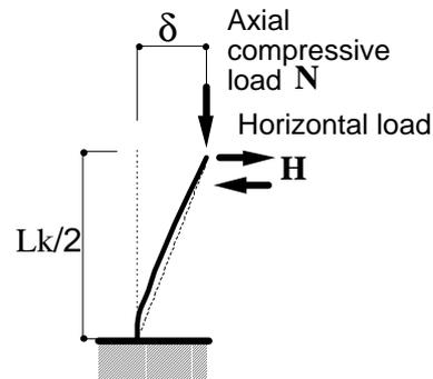
Figure 2: Loading condition (Series II)
