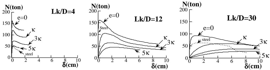
Figure 6: Axial load-lateral deflection relation (Series I: Square section)
