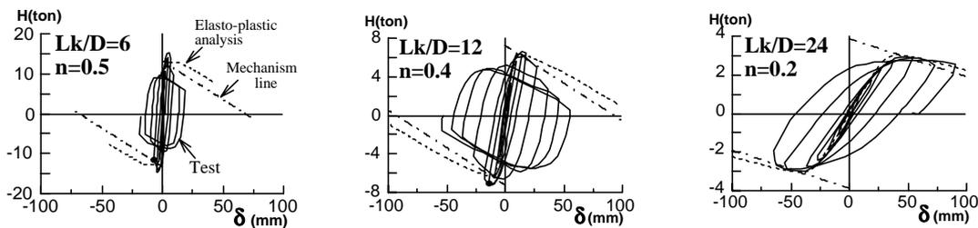
Figure 7: Horizontal load - lateral deflection relations (Series II: Square section)
