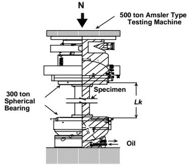
Figure 3: Loading apparatus (Series I)
