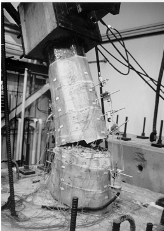
Fig. 4 - The Failure of Specimen FRG
