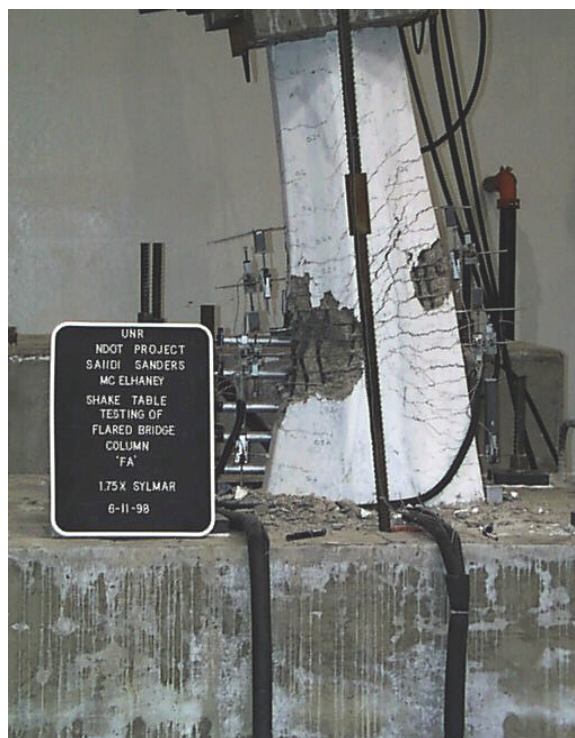
Fig. 3 – The Failure of Specimen FA
