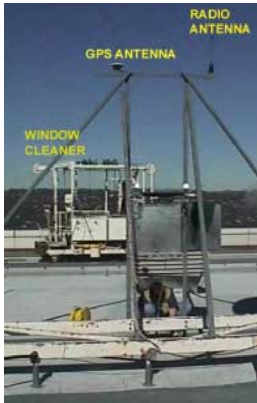
Figure 6. Deployed GPS Unit and Necessary Frame System
