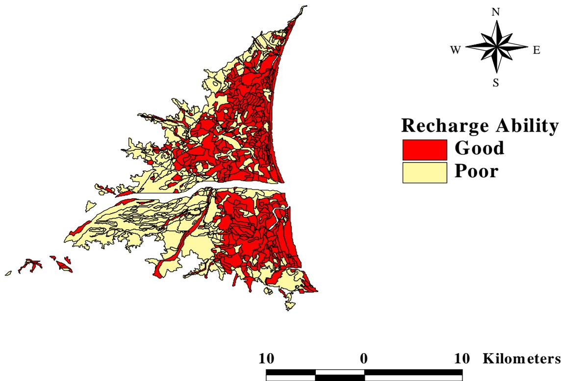
**Figure 2: The classification of recharge ability of groundwater**
