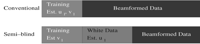
Fig. 2. Comparison of the transmission scheme for conventional least-squares (CLSE) and closed-form semiblind (CFSB) estimation.
