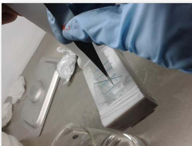
Figure 2 : Placing of substrates in Teflon sample holder.
