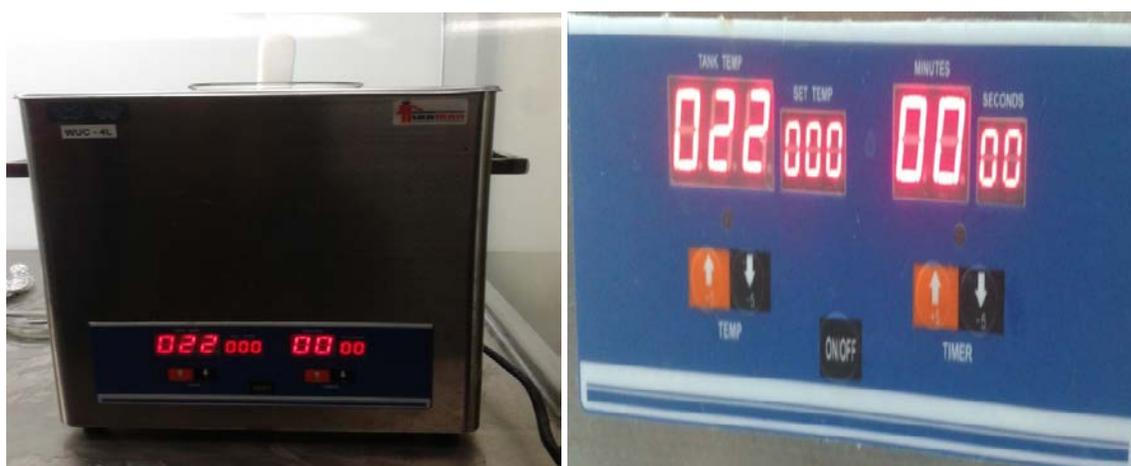
**Figure 6:** (a) substrates placed in ultrasonicator (b) magnified view of front panel from where we can set time and temperature for ultrasonication.
