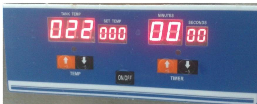
**Figure 3:** (a) substrates placed in ultrasonicator (b) magnified view of front panel from where we can set time and temperature for ultrasonication.
