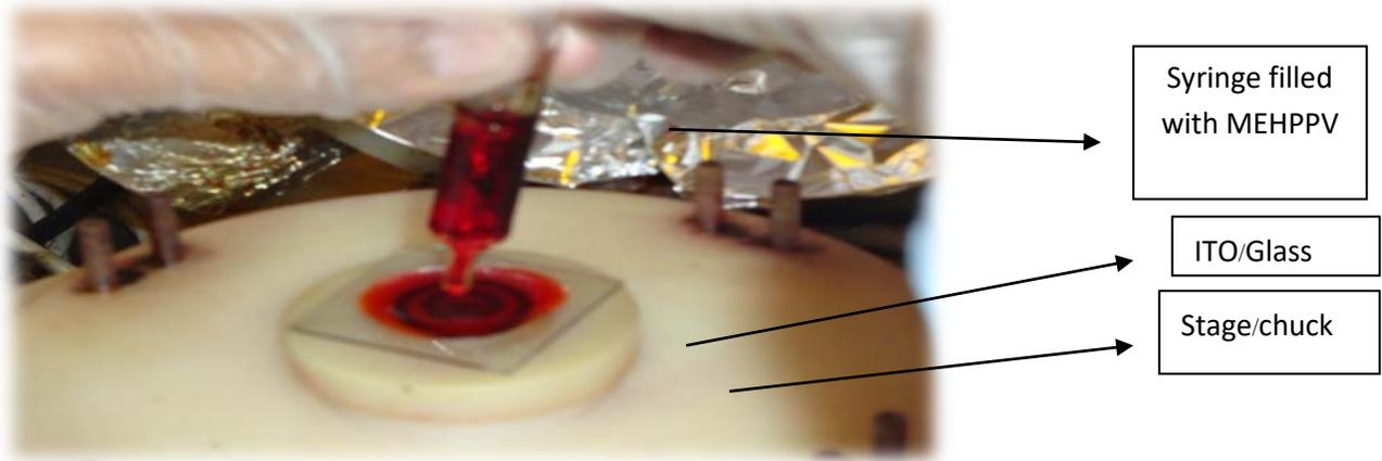
**Figure 9:** MEHPPV coating using spin coater
