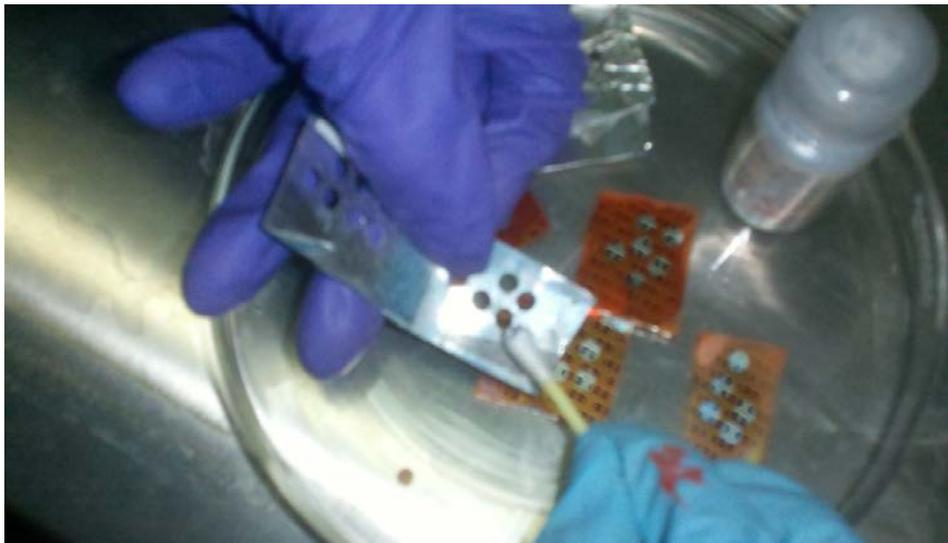
**Figure 10:** Application of Ga-In contact dots with cotton swab as cathode
