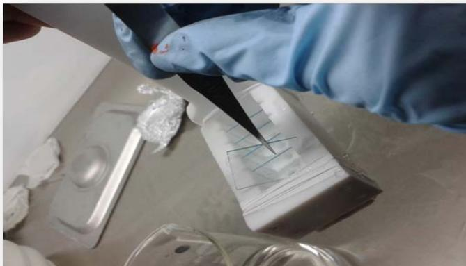
**Figure 6:** Placing of substrates in Teflon sample holder
