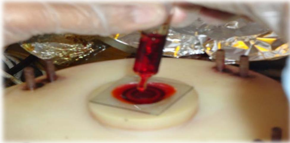
**Figure 7:** PR Coating using Spin Coater
