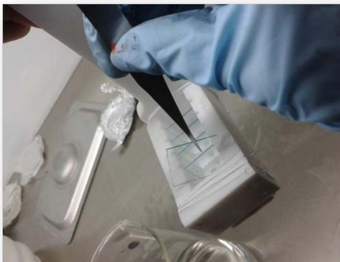
**Figure 5:** Placing of substrates in Teflon sample holder
