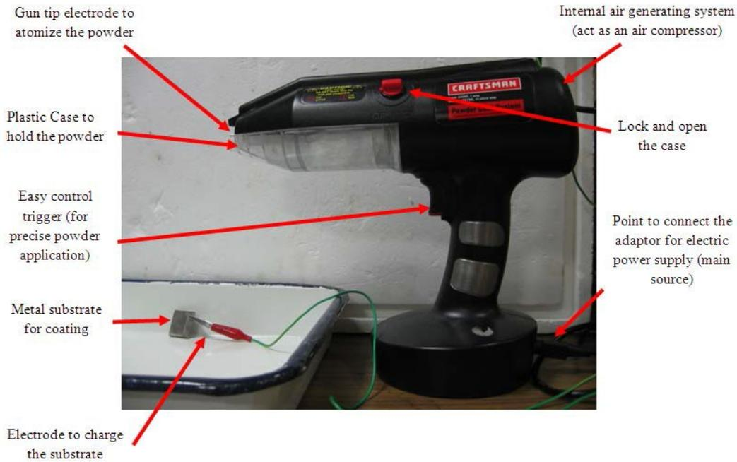
*Fig. 9.1: Electrostatic spray gun showing metal substrate for coating.*
