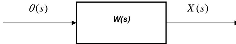
FIGURE 4-5 OPEN-LOOP SYSTEM
