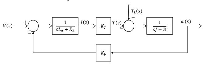
**Q2.** Design using Bode plot-based techniques a controller of the minimum order possible to control the speed of the motor for the following time domain specifications:  $e_{ss} \leq 2\%$ ,  $t_s \approx 0.5s$  ( $\pm 2\%$  tolerance band),  $\% M_p \leq 20\%$ .
