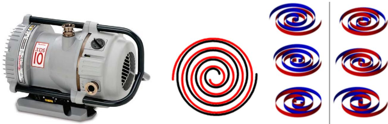
Scroll pumps are an excellent alternative to rotary vane pumps where oil free pumping is desirable. The ultimate vacuum achieved by a Scroll pump is  $1 \times 10^{-2}$  mbar.
