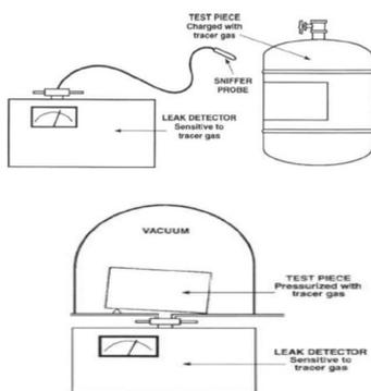
(a) In the sniffer-probe mode, the TP is filled with tracer gas and the exterior is scanned with a probe that is attached to the inlet of the leak detector. The probe continuously admits (or "sniffs") some of the air directly surrounding the TP. This air is inducted to the analytical portion of the leak detector, where any of the tracer gas that may be leaking from the TP is detected.
