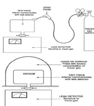
The TP (if it is of smaller volume) is evacuated directly by the leak detector. If the TP is of large volume, it is additionally evacuated by a separate vacuum pump.
