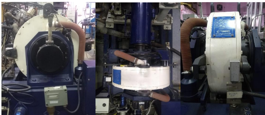
Figure 3: Eddy Current Dynamometer coupled with the test engine
