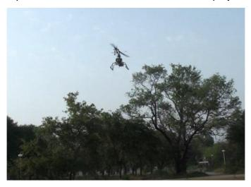
Demonstration of an autonomous mini-helicopter
