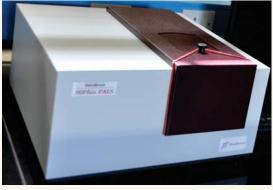
aggregation. When the potential is low, attraction exceeds repulsion and the dispersion will break and flocculate. Dynamic Light Scattering (DLS) principle can be used to determine the size distribution profile of small particles in suspension or polymers in solution. It can also be used to probe the behaviour of complex fluids such as concentrated polymer solutions.
