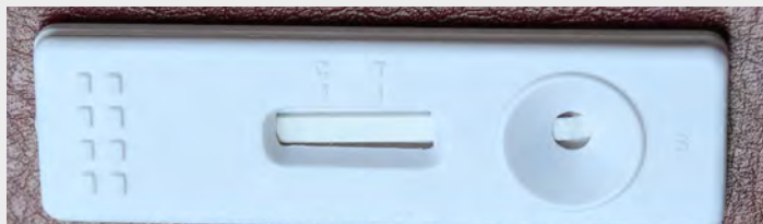
Lateral Flow Immunoassay (LFIA) Strip to detect Bovine Mastitis
