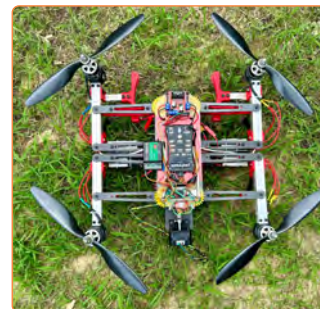
Shape-morphing quadcopter drone
