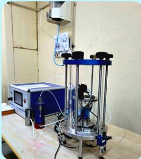
**Resonant Column Test Device** (*CHIR-AYU Controls, Model: 31-WF8600*) has been procured. The instrument is used for advanced soil testing to determine dynamic soil properties, including shear modulus and damping ratio at small strain levels, supporting research in earthquake engineering, machine foundations, and soil-structure interaction.
