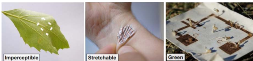
Figure. Flexible Electronics with different functionalities (from left to right): transparency, mechanical flexibility and biocompatibility.
