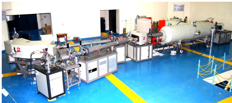
1.7 Million Volt Tandem Accelerator with beam lines for ion beam analysis and microfabrication
