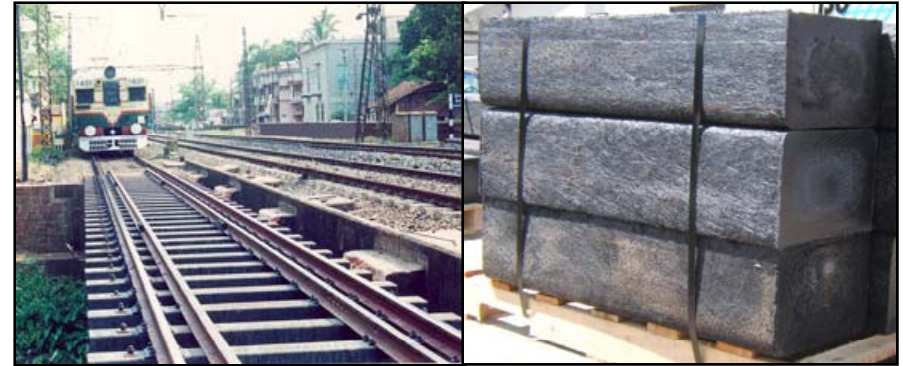
Railway sleepers with similar material from a company outside India has been tested in Eastern Railways (left); sleepers with recycled plastic from supplier staked up (right).
