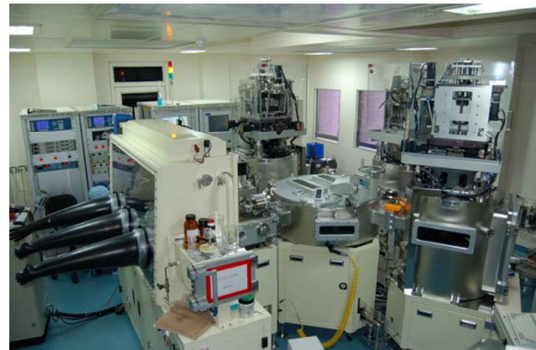
Cluster tools for device fabrication. This tool is also used to fabricate 1.5 inch passive matrix colour displays
