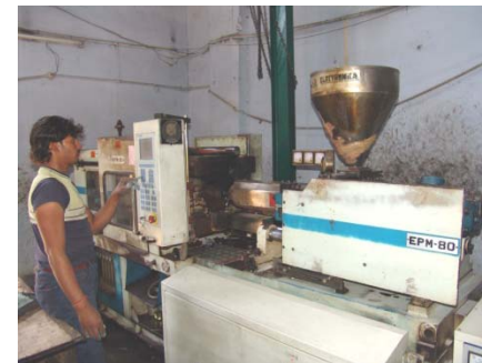
30 Kg batch process employing an Injection moulding machine at the Falcon industry-Kanpur(left) ; finished product for making dog-bone samples (right)
