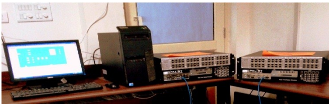
Fig. 14: Real time digital simulator test bed with master and slave control, Power systems laboratory, IIT Gandhinagar
