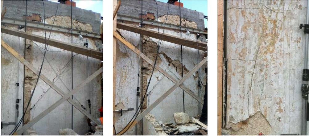
**Figure 2.4** The first two figures starting from the left represent the panel's damage at a the end of the test (positive and negative direction, respectively). On the right, cracks in the panel's extremities due to a flexural response.
