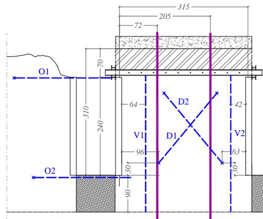
**Figure 2.3** Draft of the transducers location on the masonry tested panel.
