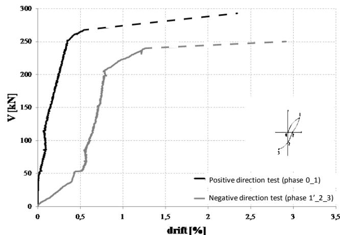
**Figure 2.5** Shear-drift curve of the two in-plane shear tests and the ideal diagram of the cyclic response.
