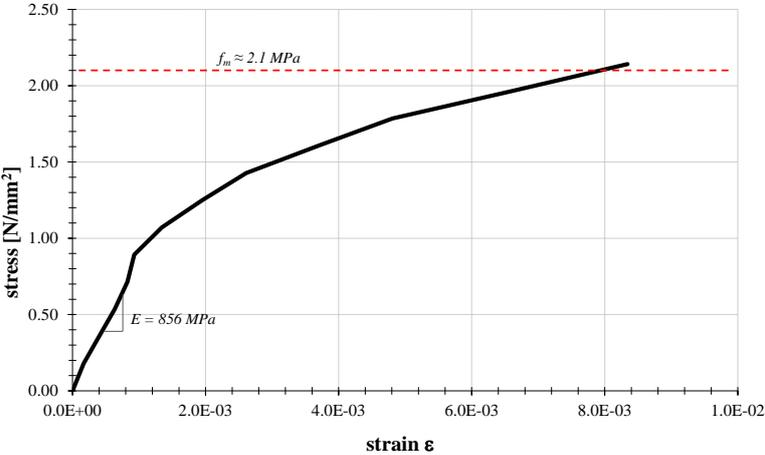
Figure 3.2 Medium strain-stress curve obtained by performing double flat jack test.
