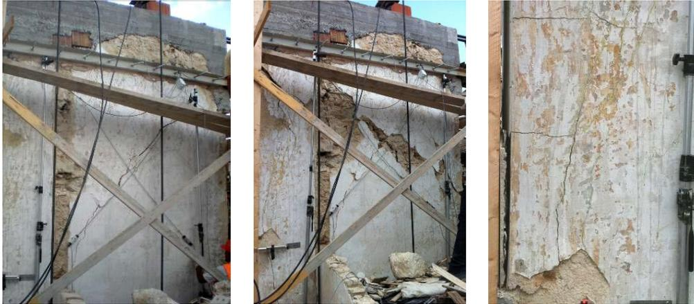
**Figure 2.4** The first two figures starting from the left represent the panel's damage at the end of the test (positive and negative direction, respectively). On the right, cracks in the panel's extremities due to a flexural response.
