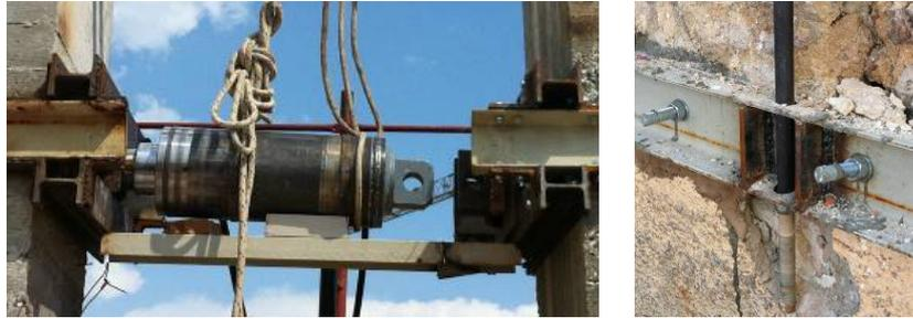
**Figure 2.2** On the left, system of the actuator's connection; on the right, connection of the steel pre-stressed bars to the UPN steel profile.
