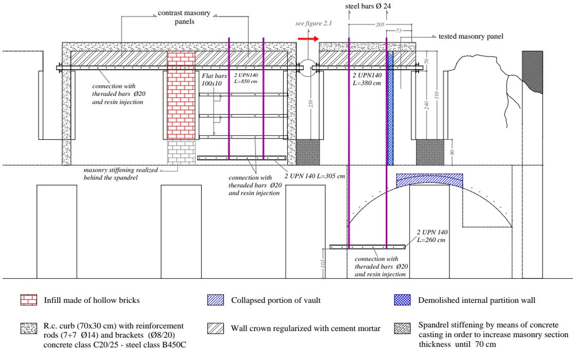
Figure 2.1 Test setup draft (the red arrow indicates positive direction of the applied load action)
