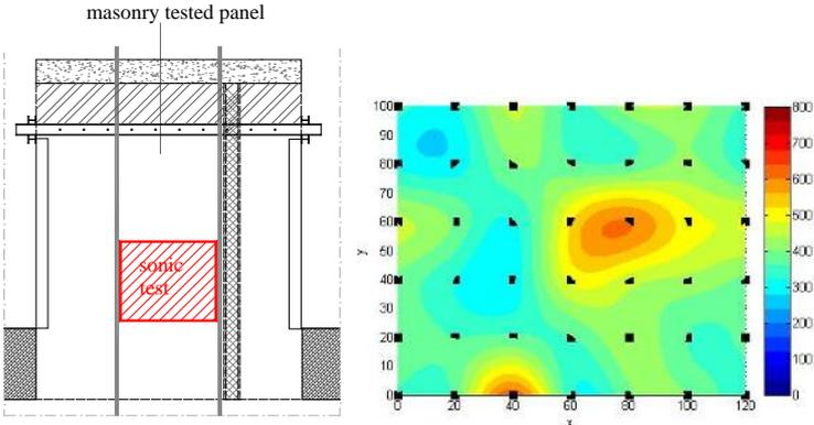
Figure 3.1 Masonry panel where sonic tests have been executed and map of the sonic pulse velocities.
