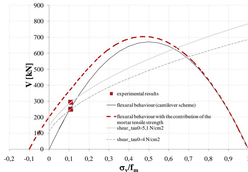
**Figure 4.1.** Comparison between resistance domains proposed in the NTC 2008 and experimental results obtained by racking test.
