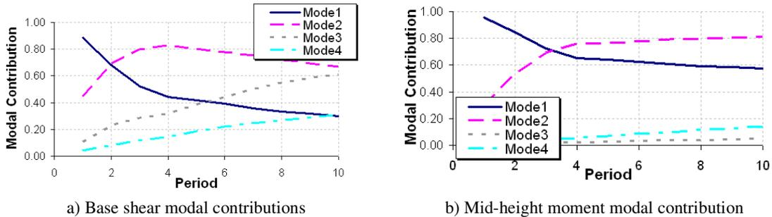
**Figure 3.** Shear and moment modal contributions for the first 4 modes in a cantilever wall
