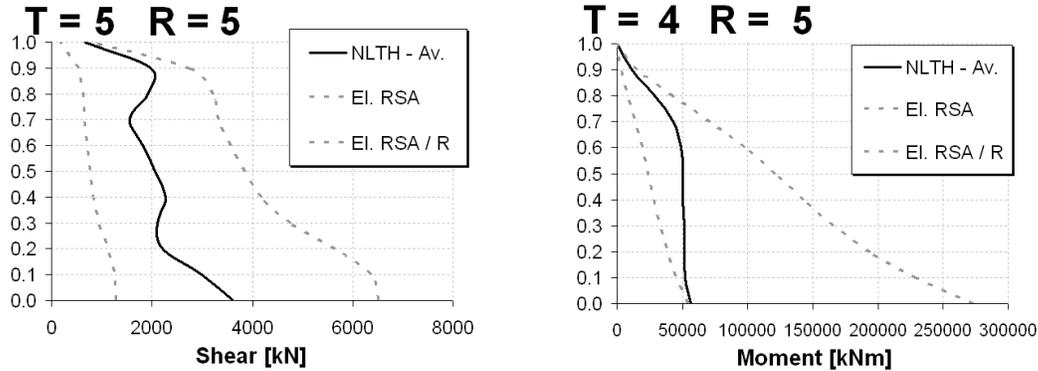
**Figure 4.** Comparison between shear and moment demand and predictions offered by elastic RSA and RRSA
