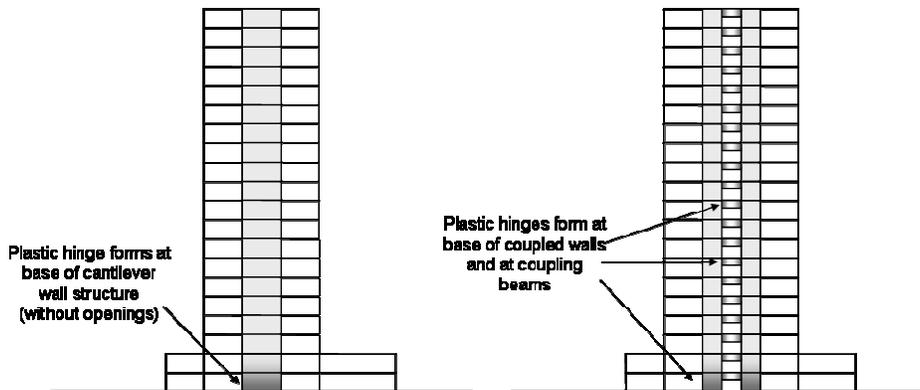
**Figure 1.** Plastic hinge locations in cantilever and couple walls.
