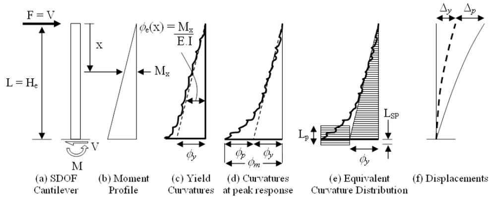
**Figure 7.** Curvature distribution in an inelastic cantilever (adapted from Paulay and Priestley, 1992)
