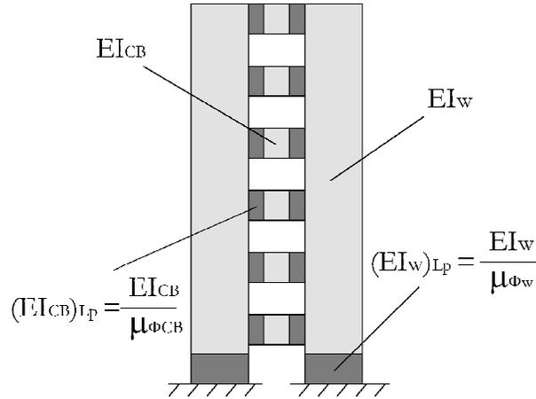
**Figure 6.** Stiffness reduction at plastic hinge locations according to the substitute structure method.
