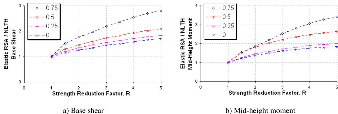
**Figure 5.** Variation of the effective reduction factor,  $eR$ , in terms of base shear and mid-height moment with the strength reduction factor,  $R$ , and the coupling ratio  $\beta$  (from 0 to 0.75).
