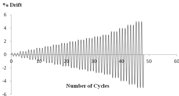
**Figure 5.** Loading history in displacement controlled mode
