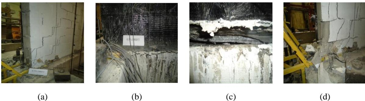
**Figure 6.** (a) Initial diagonal crack, (b) FRP sheet connected to the foundation prior to the anchor pull-out cone failure, (c) FRP anchorage failure and the separation of FRP from the foundation, (d) corner crushing of masonry
