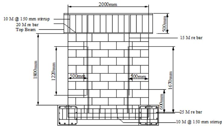
**Figure 1.** Geometric details of the masonry wall specimen
