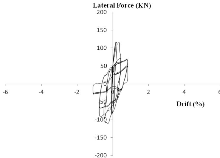
**Figure 7.** Hysteretic Load-displacement relationship for un-retrofitted companion specimen, Taghdi (2000)
