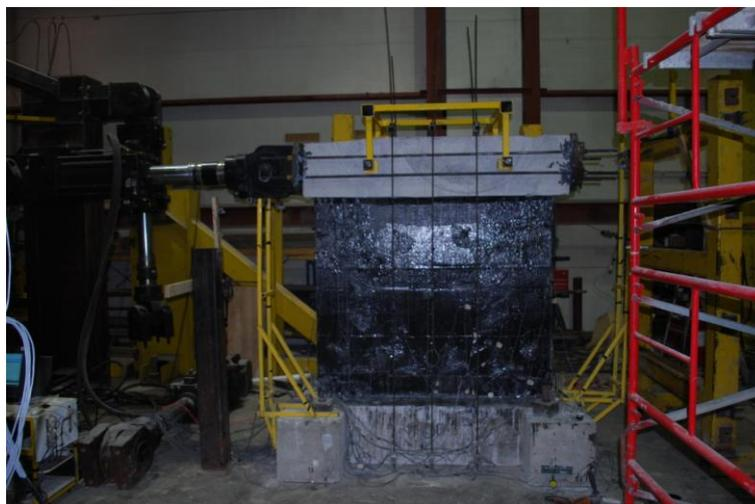
**Figure 2.** The Masonry wall retrofitted on one side.
