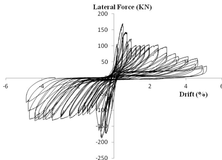
**Figure 8.** Hysteretic force-displacement relationship for retrofitted specimen.
