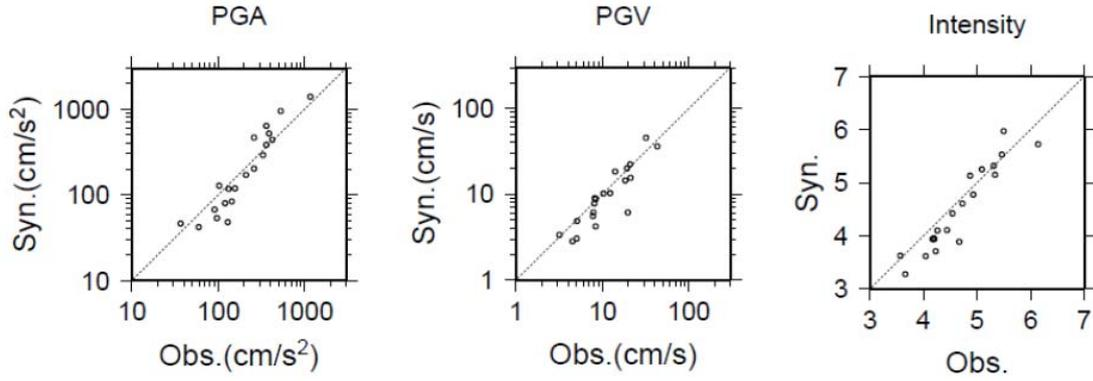
**Figure 3.1.** Comparison of PGA, PGV, and JMA seismic intensities of simulated ground motions by the average – one S.D. model (smaller fault and asperity size, i.e. larger stress drop model) to the observations.
