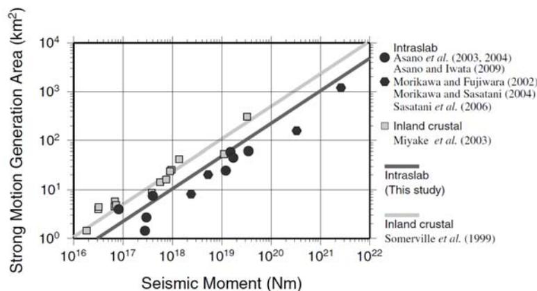
**Figure 2.2.** Scaling relationship of strong motion generation area to seismic moment for intraslab earthquakes. Circles show the strong motion generation areas for intraslab earthquakes studied in Asano *et al.* (2003, 2004) and Asano and Iwata (2009). Hexagons show the SMGAs studied by Morikawa and Fujiwara (2002), Morikawa
