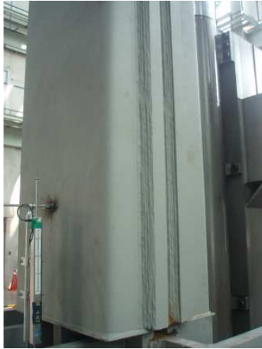
Figure 3.6. Picture for the Bottom End of the All-Steel MC-BRB After Testing
