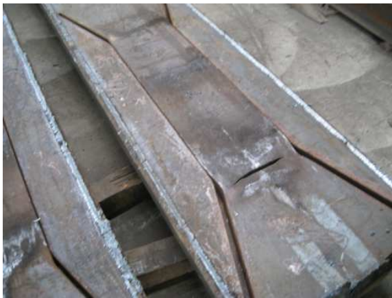
Figure 3.7. Necking and Rupture at the Bottom End of the Right Energy Dissipation Segment of the Steel Core During Tensile Loading
