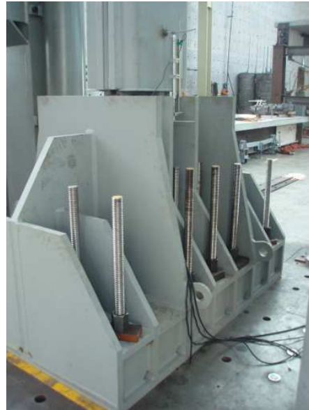
Figure 3.3. Picture for the Bottom End of the All-Steel MC-BRB Before Testing
