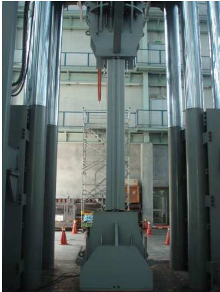
Figure 3.2. Test Set-Up of the All-Steel MC-BRB
