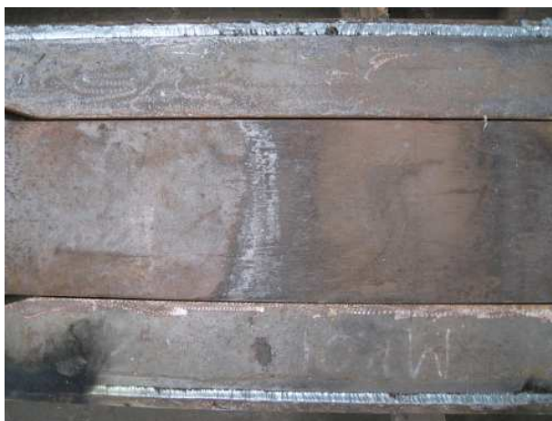
Figure 3.9. Open-up View of the Top End of the Left Energy Dissipation Segment After Testing
