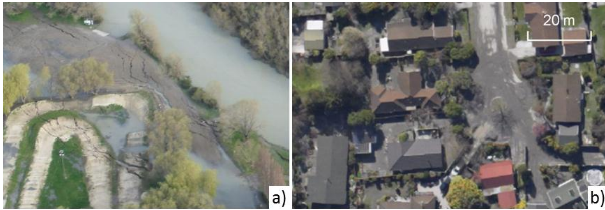
Figure 8. a) Aerial view indicating lateral spreading fissures and ejecta; b) aerial view of significant ejecta volumes north of river bend in Figure 6 (NZAM 2010)
