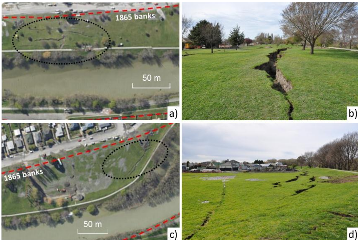
Figure 5. a) Aerial view of lateral spreading along Kaiapoi River indicating lateral spreading fissures (NZAM 2010); b) ground level view of dashed area in a); c) Aerial view of lateral spreading along Kaiapoi River indicating lateral spreading and large ejecta volumes (NZAM 2010); d) ground level view of dashed area in c)
