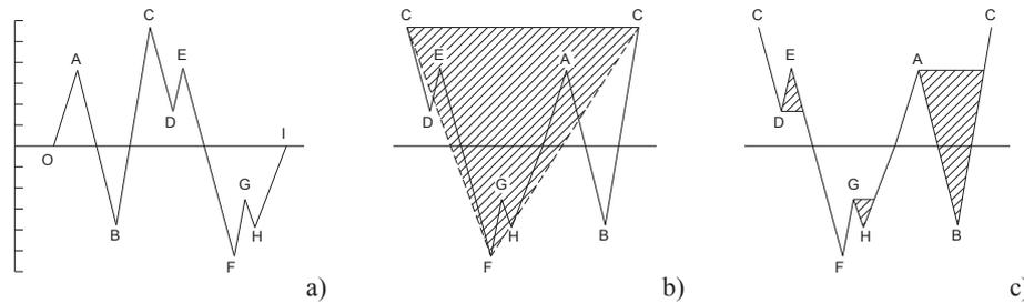
**Figure 10.** Rainflow counting method: a) random time history; b) rearranged time history and max amplitude loop (CF); c) other cycles (ED, GH, AB)
