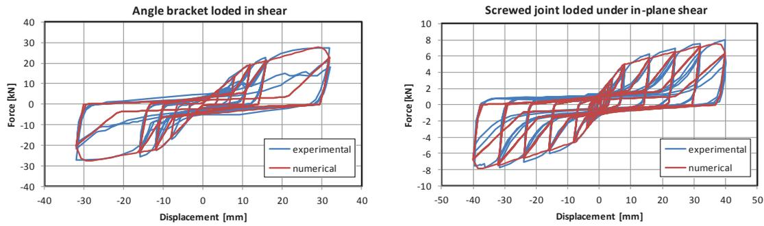
**Figure 9.** Experimental and analytical hysteresis curves comparisons
