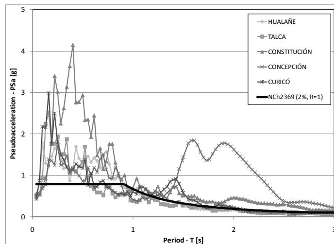
**Figure 2.** Response spectra of recorded ground motions and design spectrum from NCh2369. Of 2003, for 2% equivalent viscous damping
