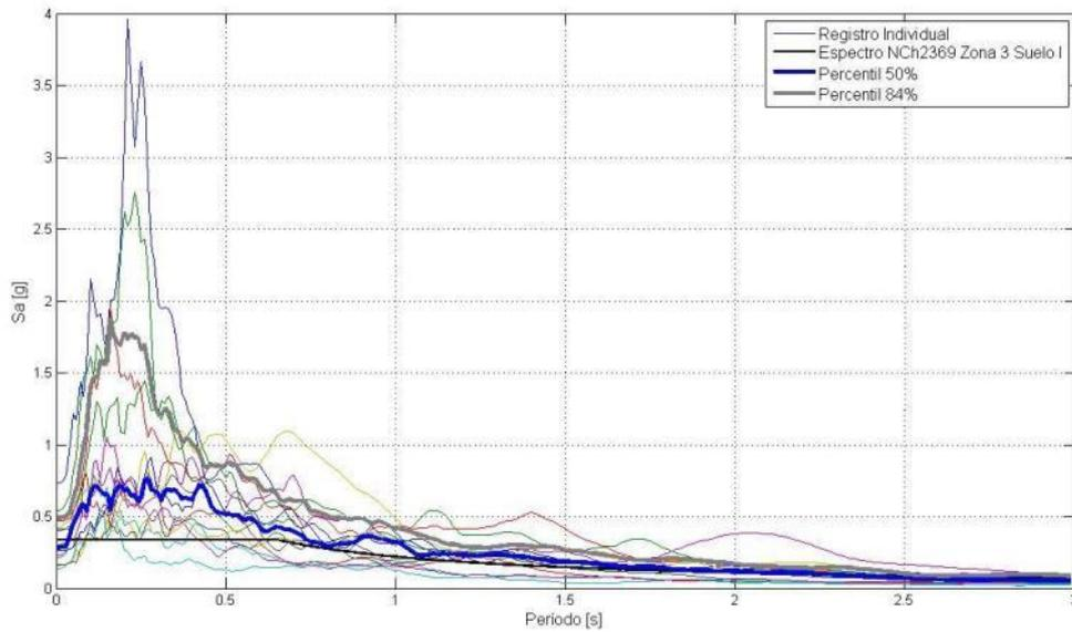
**Figure 10:** Response spectra of records used for the non linear time history analyses.
