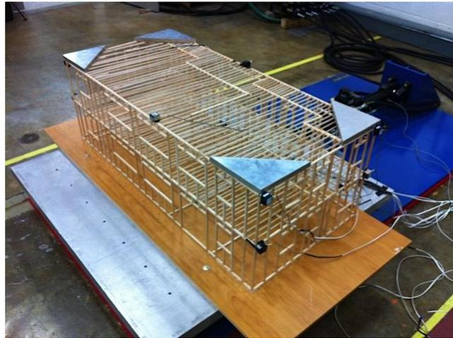
**Figure 7.** A 1/12<sup>th</sup>-scale CFS-NEES building made of balsawood.
