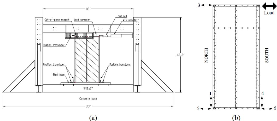
Figure 6. (a) Schematic of testing rig with specimen (b) Sensor plan where numbers correspond to position transducers measuring along the direction indicated by the arrows.
