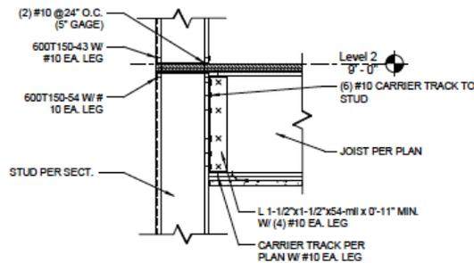
**Figure 4.** A schematic of ledger framing system.
