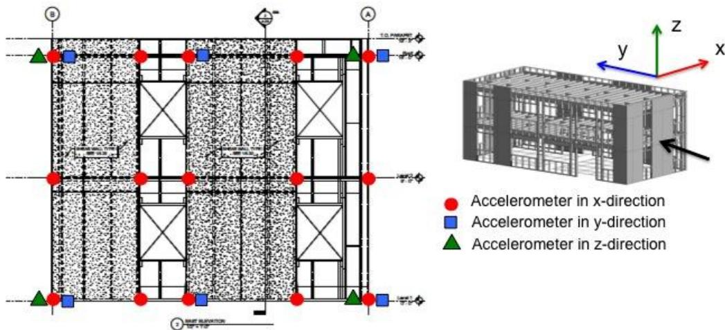
Figure 5. A sample accelerometer layout.
