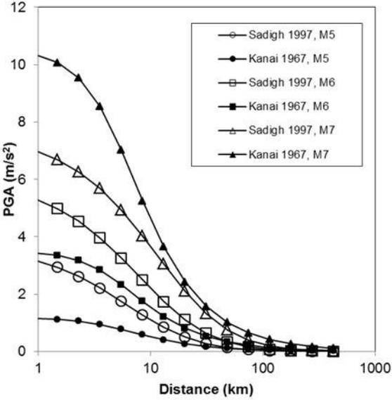
Figure 7. Comparison of ground motion prediction equations
