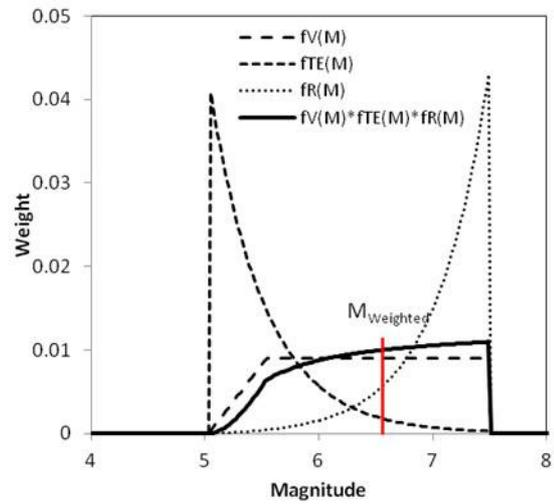
**Figure 5.** Normalized Weighting Functions for a Typical Seismic Source
