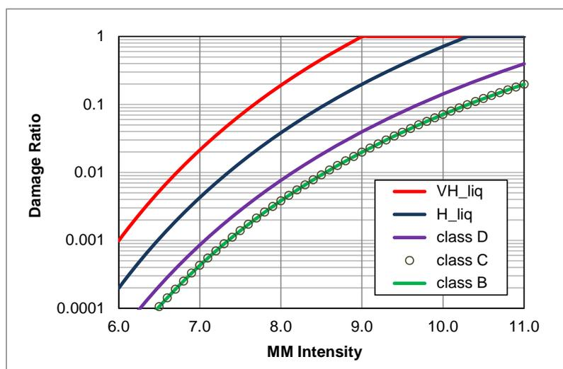
**Figure 3.** Fragility functions for brittle sewer pipes. Equivalent sets of functions were developed for potable supply, sewer, and storm-water systems, and for ductile, average and brittle pipe types.
