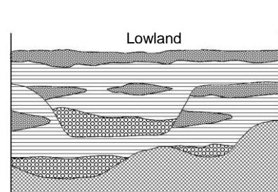
Figure 17 Geological cross-section of lowland downstream of large river in subsidence zone (schematic diagram). Example in which two glacio-eustatic cycles overlap.
