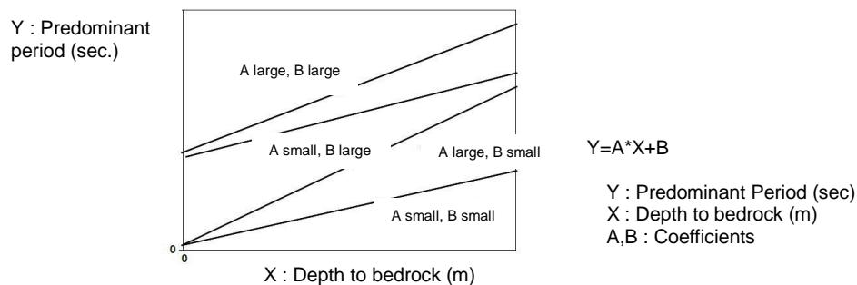
Figure 14 Schematic diagram of relationship between ground thickness and predominant period
