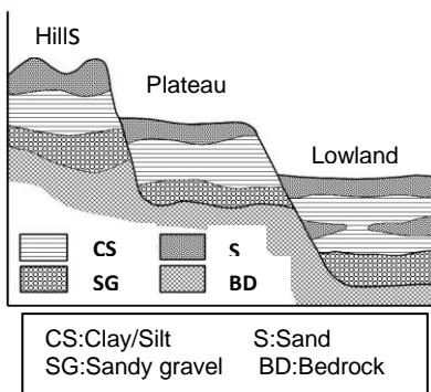
Figure 15 Geological cross-section along large river in uplift zone (schematic diagram). Example in which three glacio-eustatic cycles are recorded.
