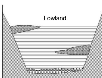
Figure 16 Geological cross-section of small valley bottom in uplift zone (schematic diagram). Example in which only deposits resulting from one glacio-eustatic cycle can be seen. Deposits are soft.
