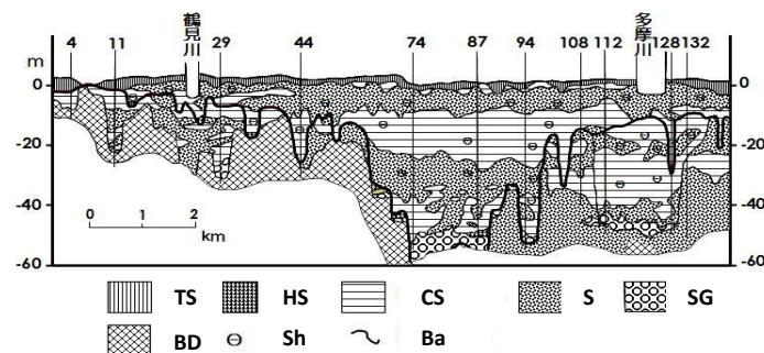
Figure 4 Geological cross-section downstream of Tama River lowlands
