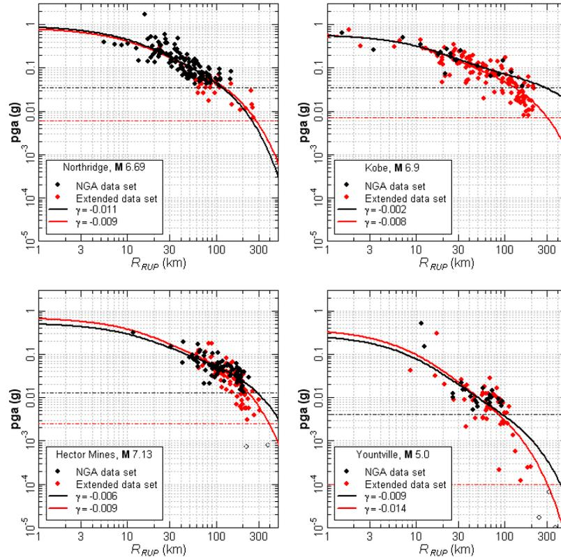
**Figure 1.** Example truncated regression fits to data for individual earthquakes (from Chiou and Youngs, 2008). Black and red horizontal dashed lines indicate the level of data truncation used in the truncated regression fitting.
