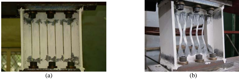
Figure 4. Failure of stiffened slit wall: (a)yielding; (b)lateral-torsional buckling
